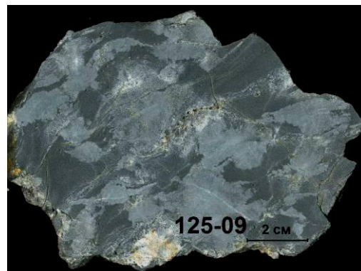
Fig. 6. Concretion ore. Light – kyanite, dark – quartz
